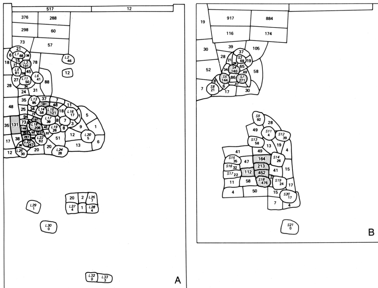
FIGURE 5: Two-dimensional polyacrylamide gel electrophoresis analysis of basic ribosomal proteins extracted from 70S ribosomes irradiated with p -azido[ 3 H]puromycin in the absence of \beta -mercaptoethanol. (A) 50S proteins. (B) 30S proteins. Areas of high radioactivity (>100 cpm) are stippled. Experimental conditions: 70S ribosomes, 2.6 \mu M; p -azido[ 3 H]puromycin, 50 \mu M, 2500 Ci/mol; photolysis time 10 min; 3500 Å lamps; counts per minute are for protein extracted from 663 pmol of subunits. Isolation: procedure A. Gel radioactivity yields: (A) 18%; (B) 18%. Note that no area corresponding to protein L21 is shown in (A). This protein is close to its isoelectric point at the pH of the first dimension and thus is only sometimes found to migrate toward the anode. A two-dimensional polyacrylamide gel electrophoresis analysis of an essentially identical experiment in which L21 was seen showed little radioactivity comigrating with this protein.
